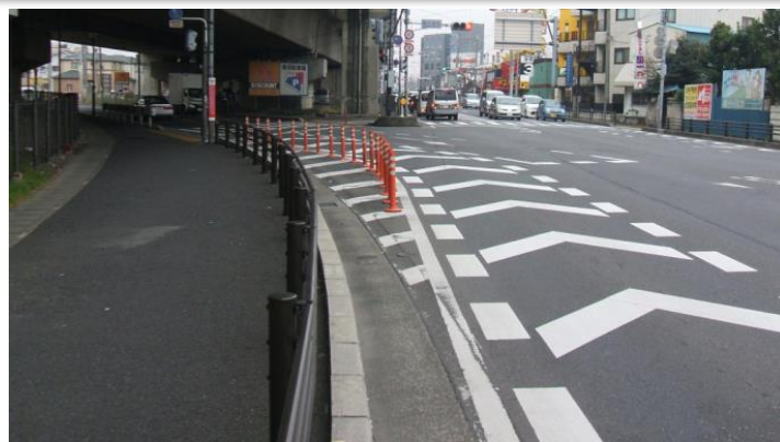
Example of placing bollards, improving the radius at the corners of the intersection
