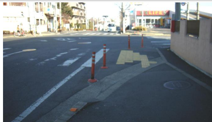
Example of placing bollards to expand sidewalk waiting space
